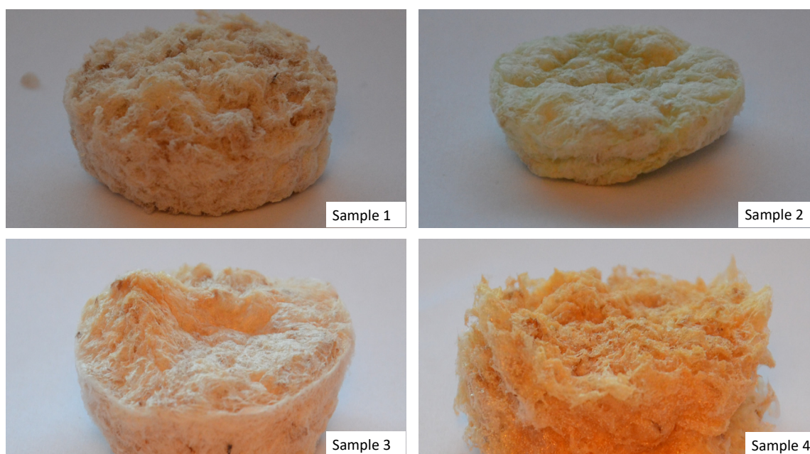
Figure 1. Prepared samples (sample 1—chitosan crosslinked with adipic and malonic acid; sample 2—chitosan crosslinked with adipic and L-glutamic acid; sample 3—chitosan crosslinked with adipic, L-glutamic and malonic acid; sample 4—chitosan crosslinked with adipic and levulinic).
