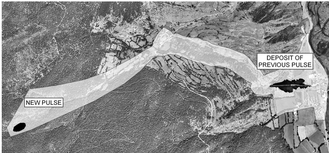
Figure 6.1: La Guingueta case. “Stop and Go” example initial conditions.
