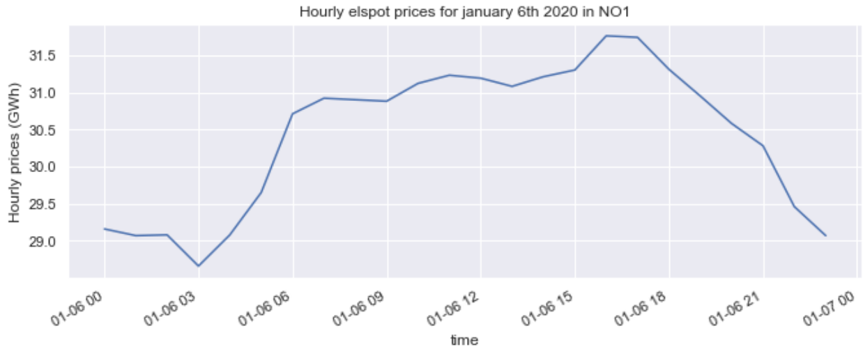
Figure 2.3 (b) Hourly prices for January 6 th , 2020. Note how the price increases in the early hours and remains sustained till evening when it goes down since people go to sleep.
