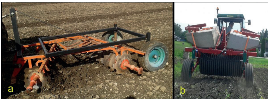
Figure B.2. Disc harrow, modified in width, frame and support wheels for depth control attached (a), and test roller I, custom built with 3-point hitch and liftable by hydraulic support wheels during transport, used with (extra heavy mechanisation) or without (heavy mechanisation) concrete load at Blæstad 2 (b).
