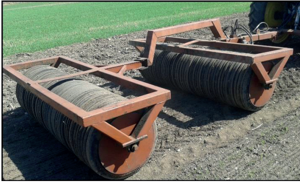
Figure B.3. Test roller II, non-liftable, used as either single (heavy mechanisation) or tandem (extra heavy mechanisation) roller at Blæstad 1 and Solør.
