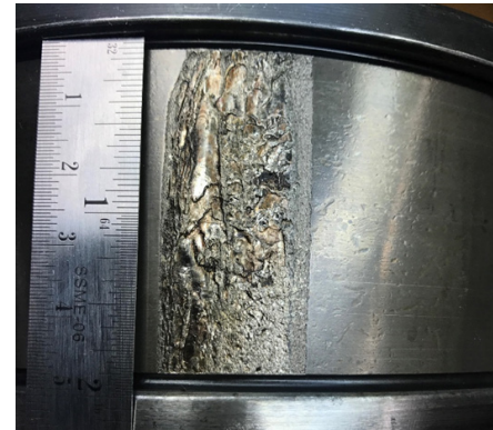
Figure 7. Post-experiment cone spall defect (ruler is in inches).
