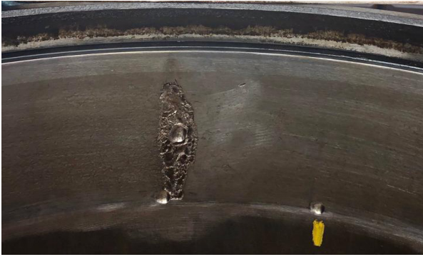
Figure 10. Initial cup spall on the bearing inboard raceway.
