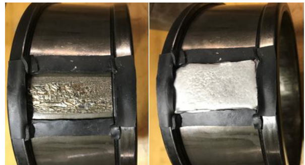
Figure 6. Casting procedure using Bismuth alloy; spalled surface outlined with tacky tape (left); Bismuth alloy cast (right).
