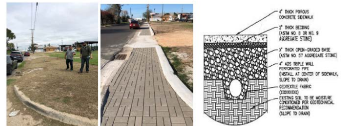
Figure 3. Before and after photos of high priority location, including engineer design of cross section of permeable pavement.
