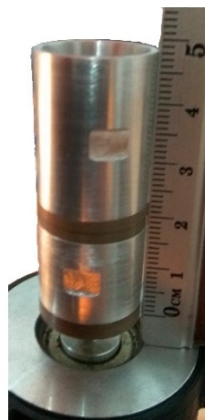
Figure 7. Prototype of the traveling wave actuator.
