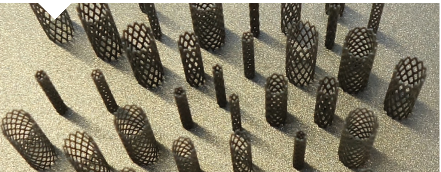
Fig. 2: Bioabsorbable Fe-Mn-C-based stent structures manufactured by selective laser melting (SLM).
