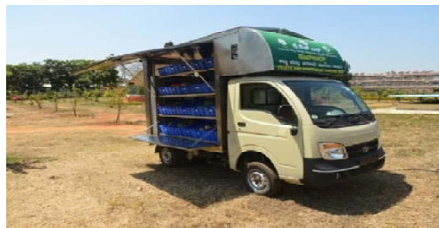
Fig. 8: a. Fruit and vegetable vending van using the solar power and evaporative cooling mechanism through misting for maintaining high RH inside the structure
