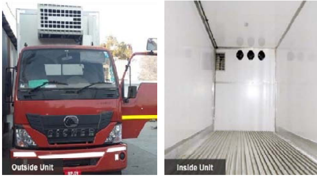
Fig. 8: b. Vending van using the Phase Change Material (PCM) for maintaining low temperature during transportation
