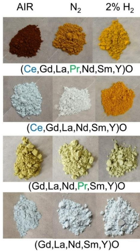
Figure 4.6. Photographs of ground sintered samples comparing the change in color with composition and sintering atmosphere.
