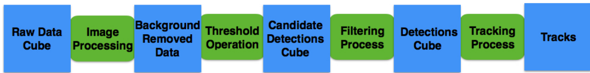
Figure 3. DBT process for detecting moving targets
