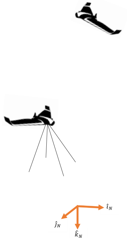
Fig. 4. An illustration of the ranging scenario used in the flight test. The upper plane has access to GPS signals, the lower plane does not. It uses autopilot sensors plus visual odometry to navigate, and then it fuses in the range to the upper aircraft. We use a common Navigation frame for both vehicles. We assume that GPS is available at the beginning of the lower planes flight to establish the common frame.
