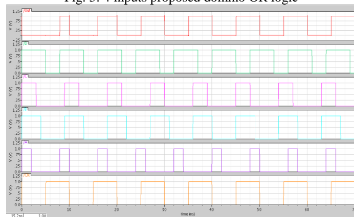
Fig. 6: Transient response of 4 inputs proposed domino OR logic
