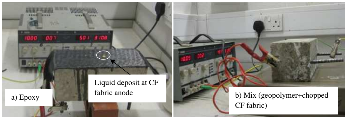
FIGURE 11: The performance of CF fabric anode bonded to concrete surface by epoxy (4.1) and CF rod anode bonded to grooved concrete by geopolymer plus chopped CF (4.2c)
