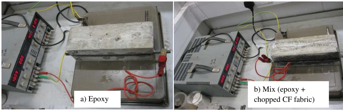
FIGURE 10: Bonding CF rod to grooved concrete prism using a) epoxy (4.2a) and b) epoxy plus chopped CF fabric (4.2b)
