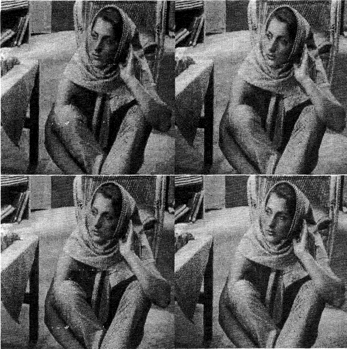
Fig. 12. Reconstructed versions of image "Barbara": (top left) using DCT at 0.25 b/pel; (top right) using a GenLOT with N = 6 (design #6) at 0.25 b/pel; (bottom left) using DCT at 0.4 b/pel; (bottom right) using a GenLOT with N = 6 (design #6) at 0.4 b/pel.
