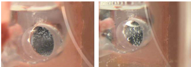
(a) Vapor bubbles onset (b) breathing vapor on the CPS wick
