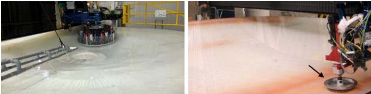
Figure 5. Large mirrors are polished with a variety of tools including the stressed lap shown polishing the LSST tertiary mirror on the left and a rigid conformal tool working one of the GMT segments shown on the right.
