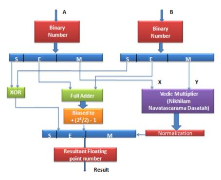
Fig. 3 Block Diagram of Universal Multiplier
