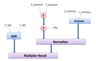
Fig. 1 Block diagram of Floating Point Multiplier
