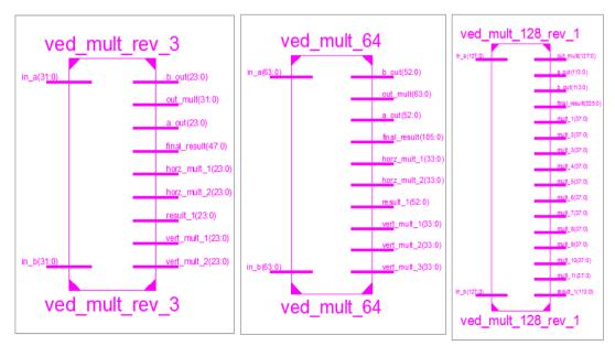
Fig. 6: RTL schematic for single, double and quadruple precision multipliers
