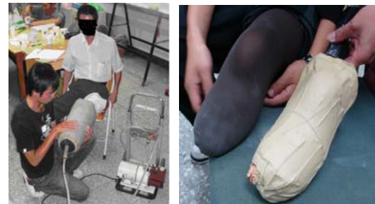
Figure 5. DUPLICATING A STUMP MOLD USING A SELF-DEVELOPED FORMING TOOL.
