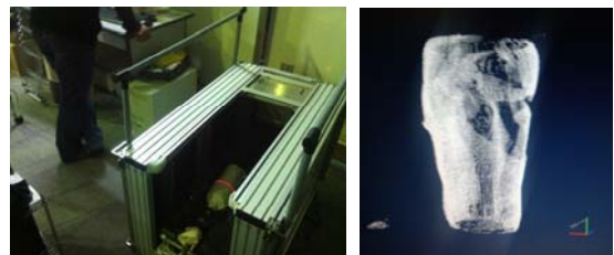
Figure 6. USE OF A SIMPLE SCANNER AND A DIGITIZED STUMP MODEL CONSTRUCTED.
