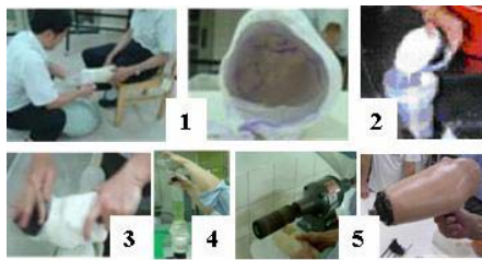
Figure 2. THE STEPS OF FABRICATING A PTB SOCKET.
