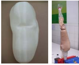
Figure 10. AN RP SOCKET MOLD AND USE FOR LAMINATION.
