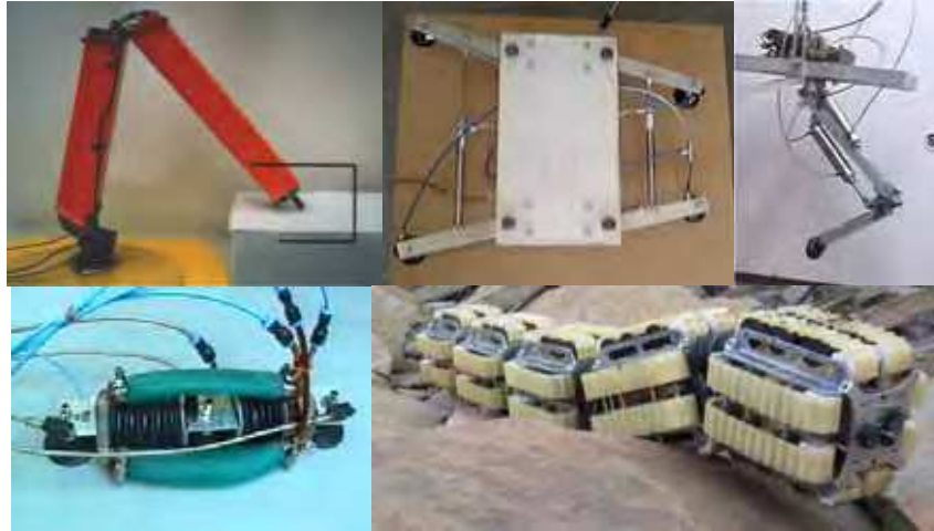
Figure 1. We contributed in these robots: (from top left) TM44 manipulator for climbing robot Robug III, Spike Junior – climbing robot, jumping leg, bellows driven crawler, OmniTread - serpentine robot developed at UofM
