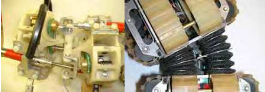
Figure 25. Joints of serpentine robots: OmniPede the predecessor of OmniTread with pneumatic cylinders (left), Integrated Joint Actuator in OmniTread (right)
