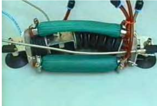
Figure 22. Robot Catty during turning procedure, muscle in first plane and bellows on the right are activated
