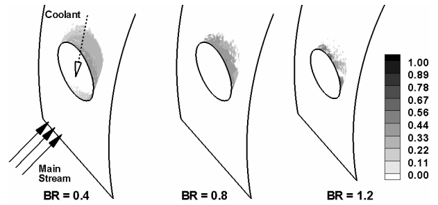
Figure 11. Impact velocity of 5 micron erosive particles
