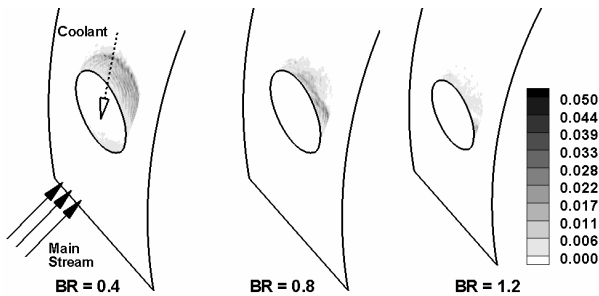
Figure 9. Percentage of 5 micron erosive particle in the coolant hole (out of all 5 micron particles)
