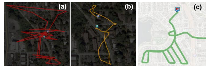
Figure 5. (a) The direction change frequency trip filter correctly filters this erroneous trip (in red). (b) The trip would not have been eliminated via the centroid-based trip filter (shown in orange). (c) Even a very "turny" legitimate trip like that in (c) is not erroneously filtered, which has a direction change ratio of 0.19 and 0.33.
