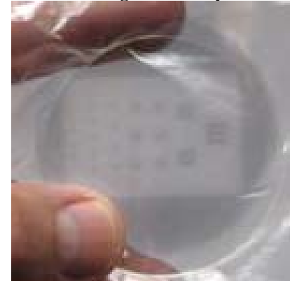
Figure 2. Vision test through 4mm acrylic lens and four .05mm layers of polyethylene
