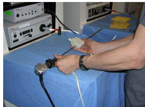
b. Endoscope and shielding device upon assembly
