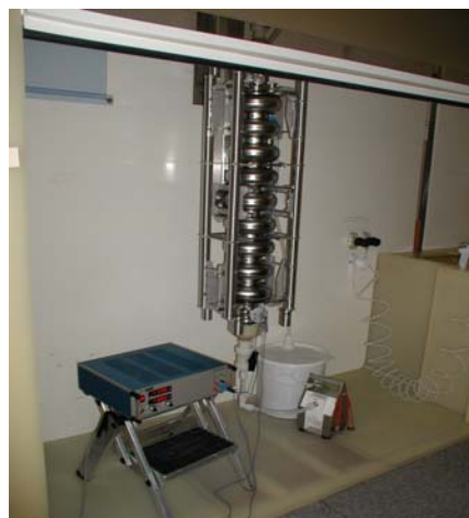
Figure 8: Test apparatus to anodize the cavity for test of surface cleaning by oxi-polishing at DESY
