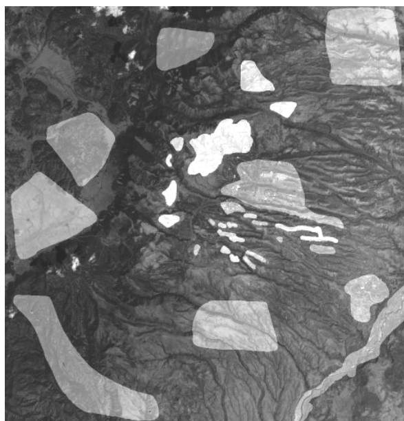
Figure 3. Training Data over Landsat imagery: White patches mark “burn” regions. Gray patches mark “non-burn” regions. Note: this image is presented at a larger spatial scale than Figure 2.
