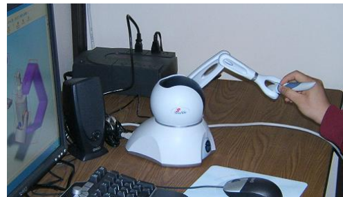
Figure 1 Virtual Environment with Haptic Interface at Lamar [Zhu 2006]
