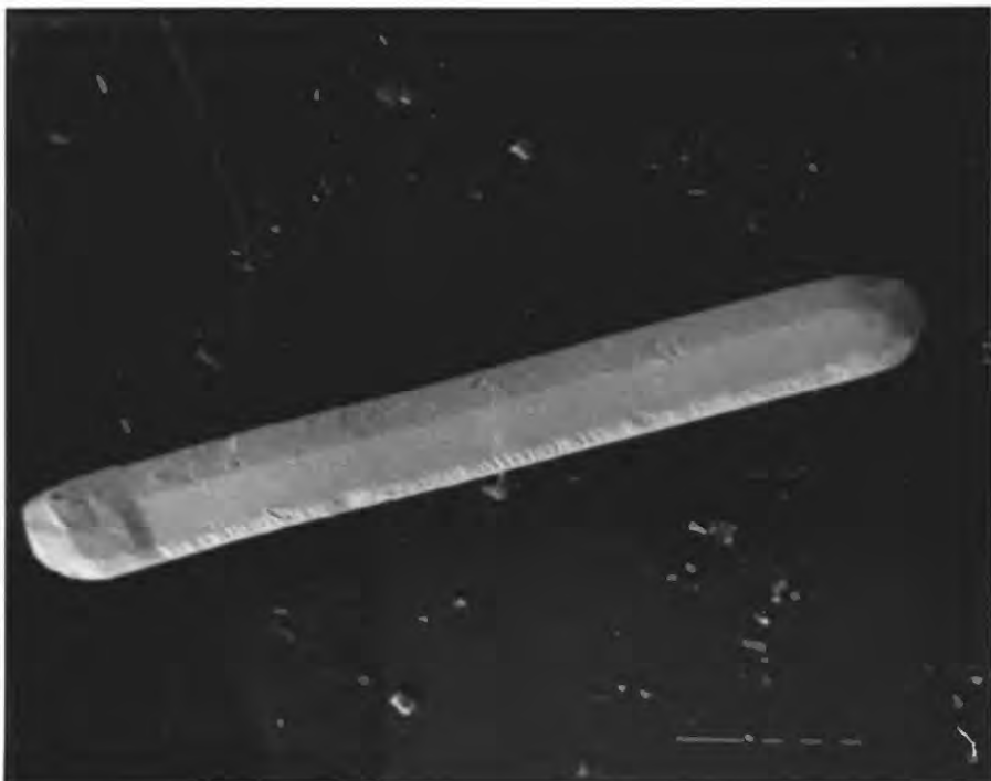
Figure 2.--Crystalline gold from the Lillian Creek placer deposit: a . spike; b . pseudo-hexagonal plate; and, c . pseudo-hexagonal rod. Scale bar equal 10 \mu\text{m} .
