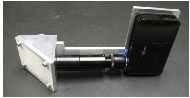
Fig. 4. The AR system detached from the surgical microscope.
