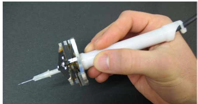
Fig. 1. Micron, a handheld micromanipulator.
