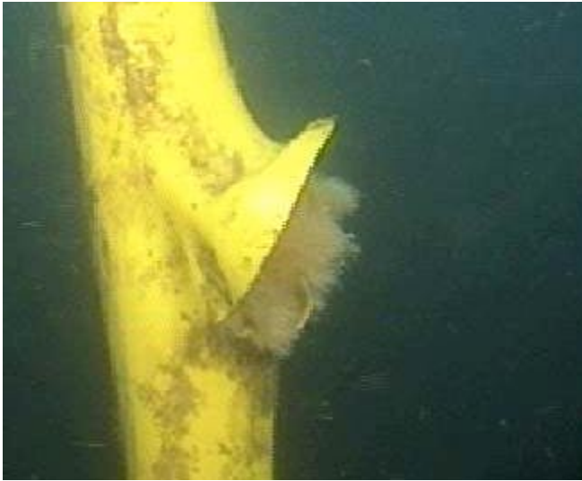
Picture 2. Outher sheath burst due to blocked annulus vent
