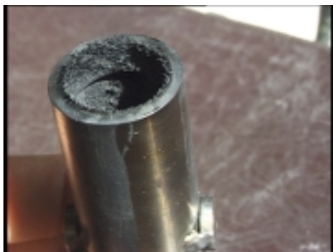
Fig 7.b. View of the exit of vaporization tube of the injector. P=3 bars and T=415 °C
