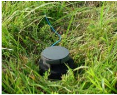
Figure 6. The Acoustic Surveillance Unit (ASU), 28 a joint development project with Signal Systems Corporation. The unit houses the VLSI wake-up and localization processors and in field tests has demonstrated detection and localization performance on par with state-of-the art DSP systems at a mere fraction of their size and power dissipation.
