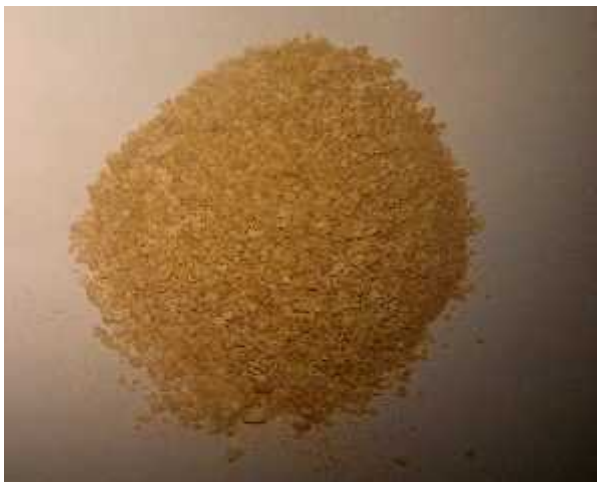
Figure 3: Pale yellow Crystals of L-Lysine obtained after recrystallization of crude brown Lysine crystals
