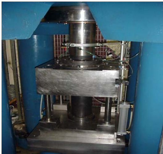
Fig. 4 Tooling Assembly Setup for Fabricating the NLC Copper Disks (shown in Fig 7) and Hollow Cylinders (shown in Fig. 8) CDC Press Operating Characteristics:
