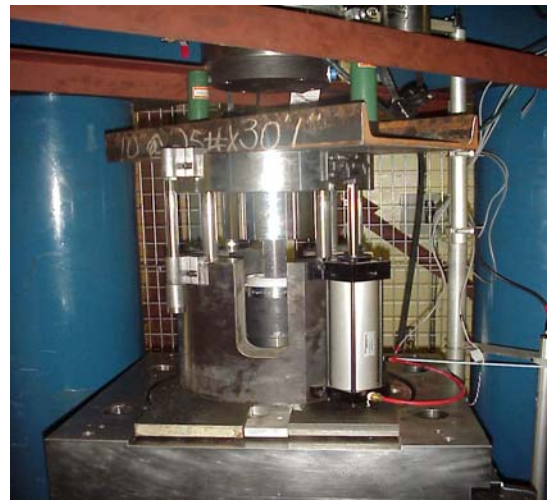
Fig. 4 Tooling Assembly Setup for Fabricating the NLC Copper Disks (shown in Fig 7) and Hollow Cylinders (shown in Fig. 8) CDC Press Operating Characteristics:
