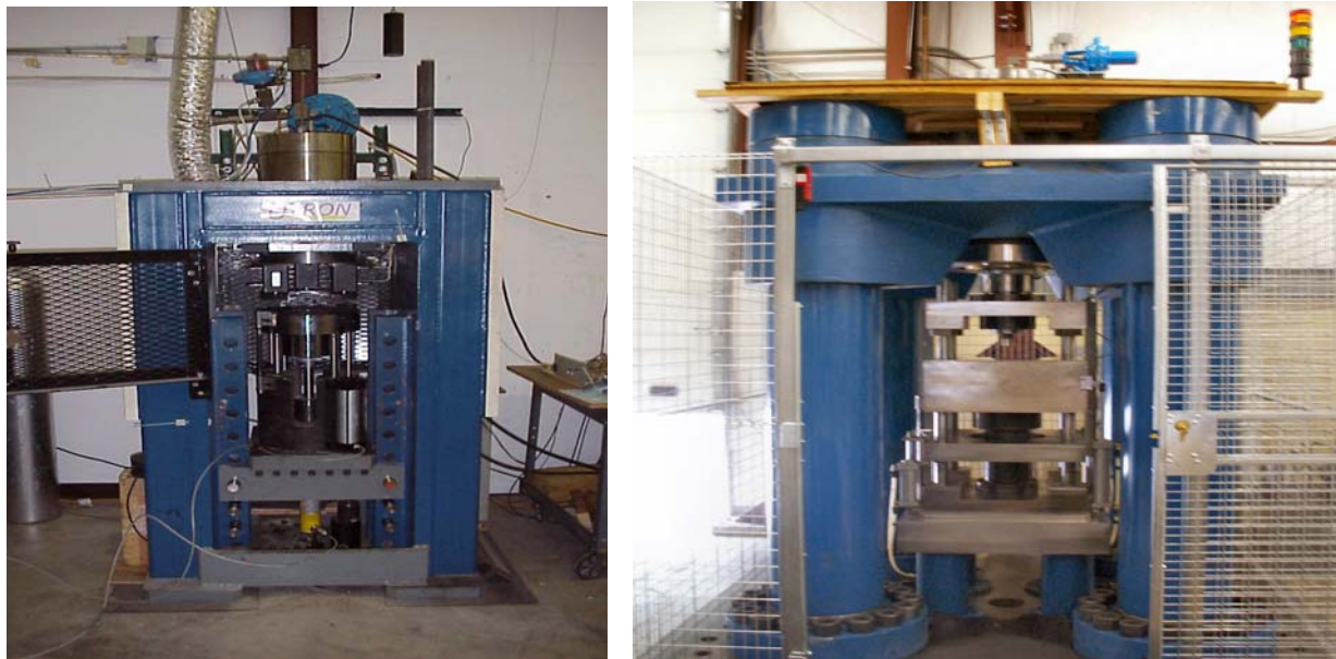
Fig1. a) 300 Ton (left) & b) 1000 Ton (right)-Combustion Driven Compaction-CDC Presses
