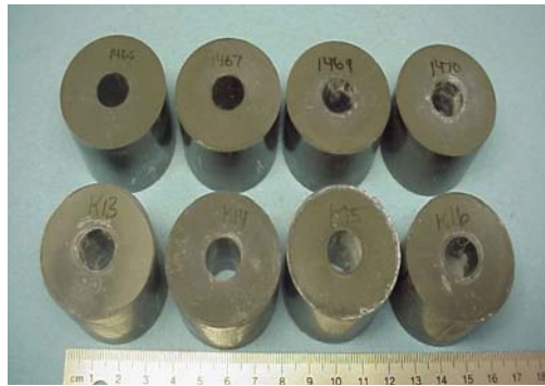
Fig. 7 Next Generation Linear Collider Copper Disks Using 1000 Ton CDC Press [12-13]
