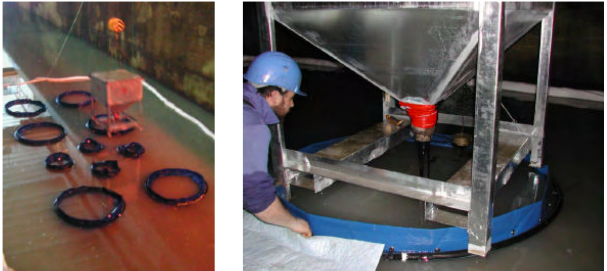
Figure 2: (left) The ten patches on the sand floor, before oil filling and water flooding. (right) Filling of an oil patch.
