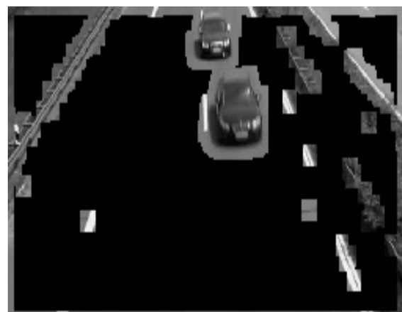
Fig.2. object detection using frame difference method
