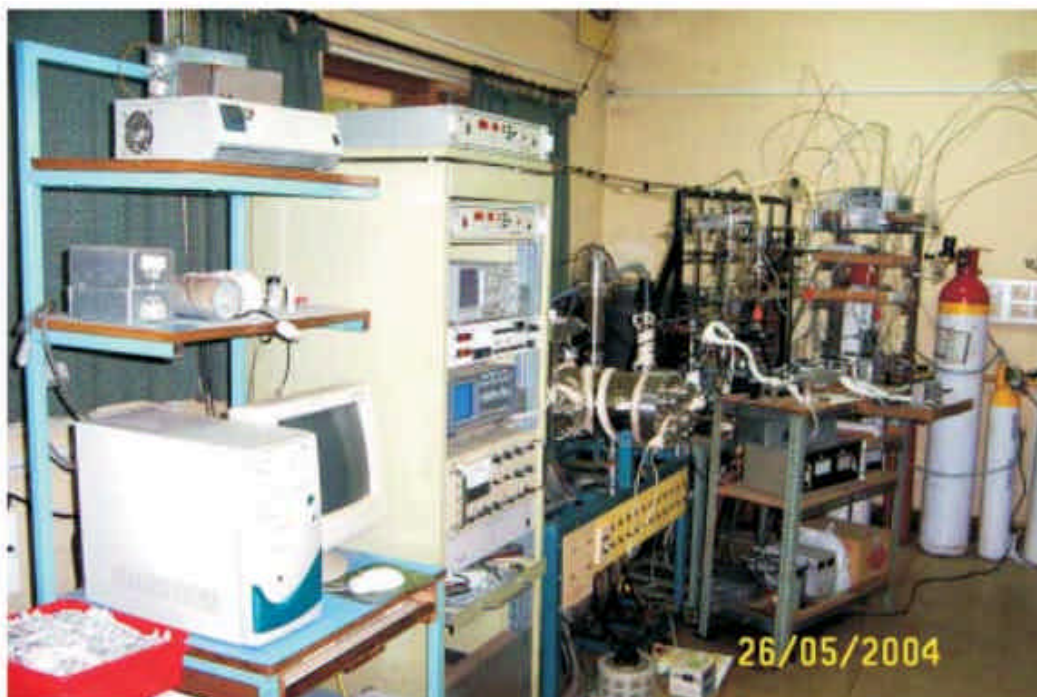
Figure 2. TPR instrument for catalysis studies.
