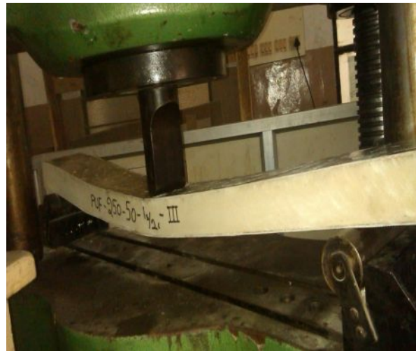
Fig 2: Specimen under three point bending test
