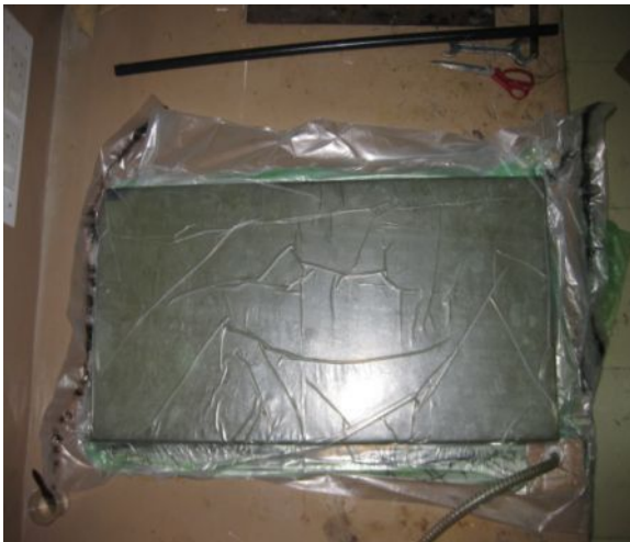
Fig 1: The vacuum bagging technique
