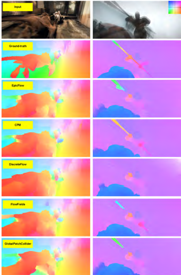
Figure 4. Qualitative comparisons among top-5 algorithms on Sintel optical flow benchmark. Top to bottom: input image (average of two), ground-truth, EpicFlow [26], CPM, FlowFields [1], GlobalPatchCollider (ours).
