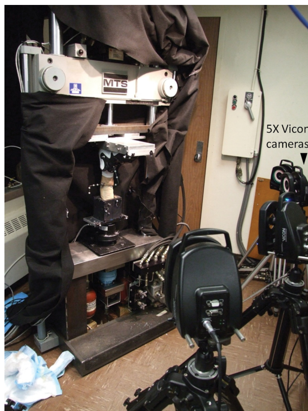
Fig. 3 Testing setup. Five-camera Vicon motion capture system (showing only four cameras) and one video camera (not shown) were used to track motions of the talus relative to the tibia.
