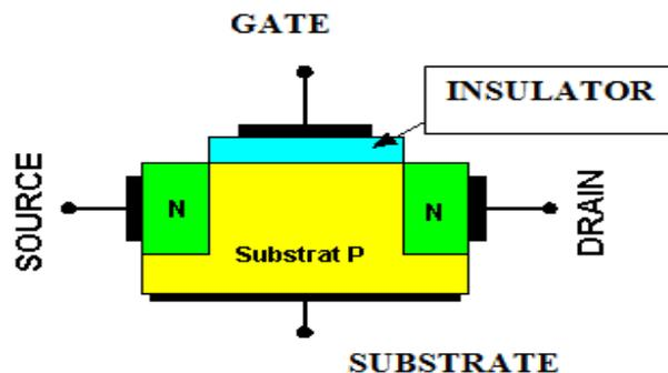
Figure 1 : Structure of the Used Transducer [2].
