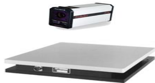
Fig. 2 Measurement equipment (motion capture camera and force plate)
