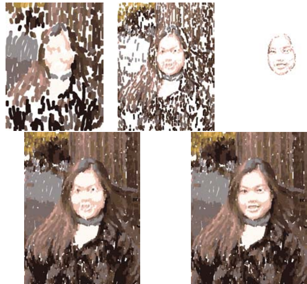
Fig. 6 Visual feedback painting with object segmentation (subject's face here). The first row shows each hierarchy, and the second row shows the overall result.
