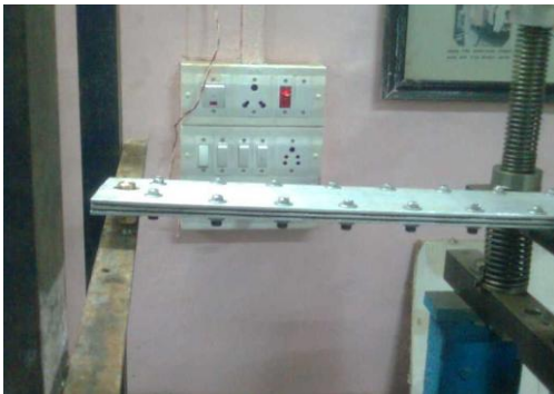
Fig.2(a). Prepared MR Fluid Sandwiched beam
