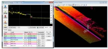
FIGURE 9. BREAK LINE EXTRACTION IN TOPODOT: CROSS SECTION VIEW (LEFT) AND ISOMETRIC VIEW (RIGHT)
