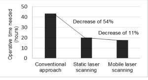
FIGURE 13. OPERATIVE TIME NEEDED FOR EACH METHOD TO ESTABLISH AN URBAN SURVEY FOR A SECTION OF 300 METERS LENGTH (SCALE 1:200)
