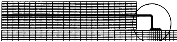
mesh of a solder joint
