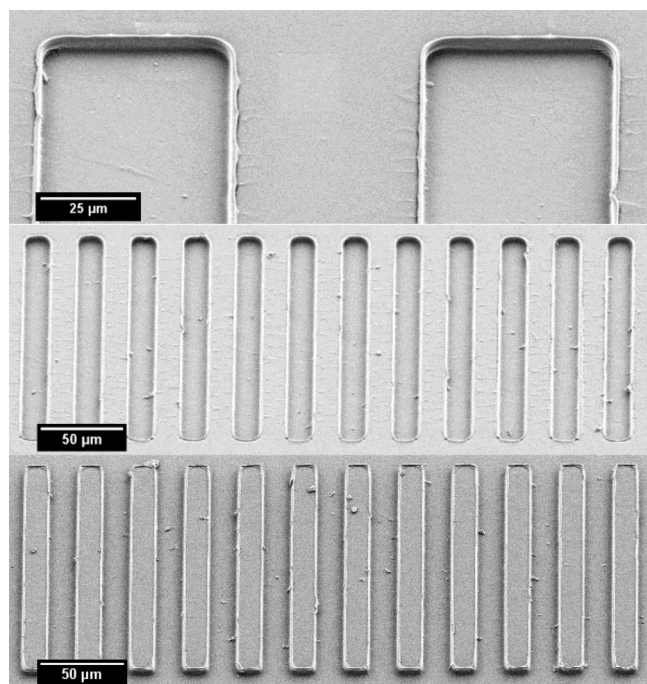
Figure 10. SEMs of 50 \mu\text{m} trenches (top), 16 \mu\text{m} trenches (middle), and 16 \mu\text{m} hills (bottom).
