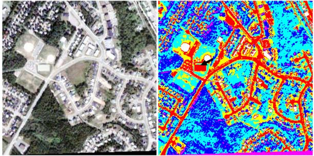
**Figure 3.** A typical output of the *k*-means algorithm from Quickbird MS imagery: (left) original true color composite ortho-image; (right) segmented image with the road cluster shown in red. The black arrow points to an example of misclassifying other spectrally similar objects as roads.
