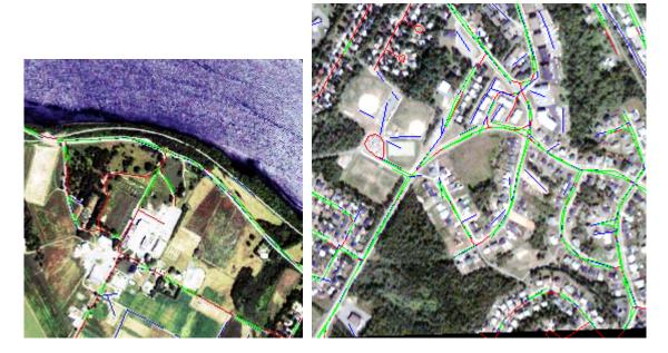
Figure 7. Results evaluation for the Ikonos test image (left) and the Quickbird test image (right): Green – correct extraction, red – missed roads, blue – false extraction
