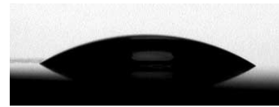
(a) Water droplet on the silicone surface
