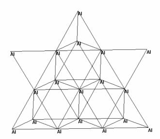
Fig.1.Two layers of Al-surface formed by 18 atoms on (111) crystal plane .
