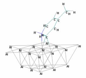
Fig.3. Adsorption protonated pyridine derivative at the Al-surface in acidic media.
