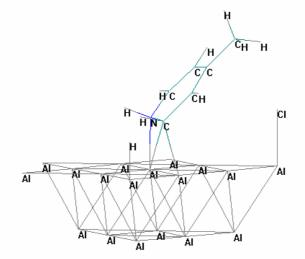
Fig.4. The co-adsorption of protonated pyridine derivative with H<sub>d</sub> and Cl.
