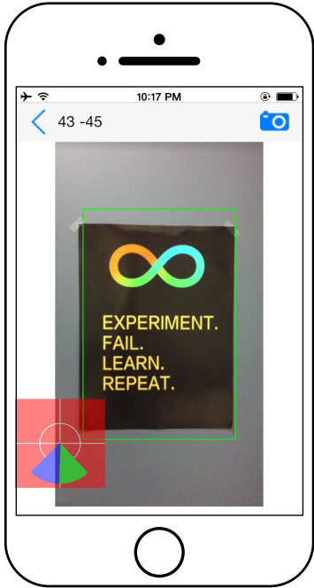
Figure 3. The capturing interface. The green guiding box is specified by the host for adjusting the size and position of the object. The compass in the bottom-left corner shows the angular distribution of all the cameras. The numbers in the top-left corner show the angle values between neighboring cameras for fine position tuning.
